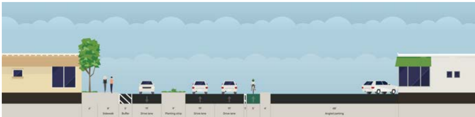
Figure 6.3-6: Class II Bike Lane along Northbound San Dimas Avenue (Arrow Highway – Railroad Tracks)
